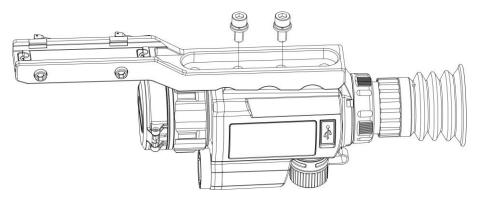
Figure 2-6 Install Screws
