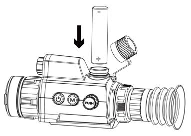
Figure 2-3 Install Battery
