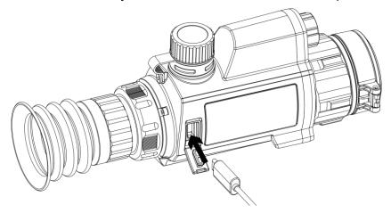
Figure 2-1 Cable Connection
