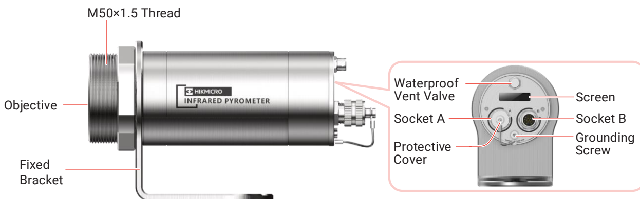
Figure 1-1 Pyrometer Exterior Components
