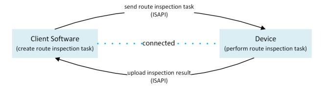
Figure 5-1 Route Inspection Work Flow
