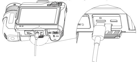
Figure 2-1 Charge Battery via Type-C Cable
