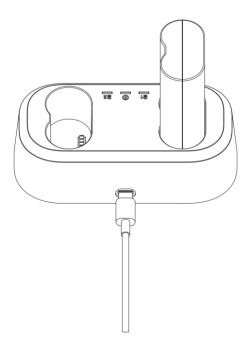
Figure 2-2 Charge Battery via Charging Base
