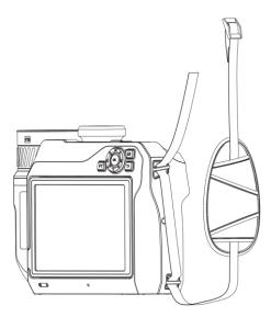
Figure 2-4 Thread Hand Strap Through Attachment Points
