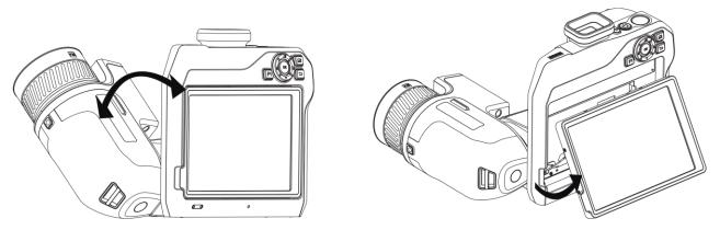
Figure 2-11 Tilt Lens and Screen
