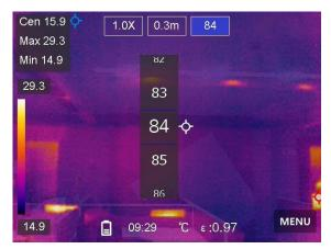
**Figure 3-3 Adjust Optical-Thermal Ratio**
