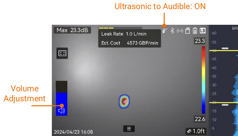
Figure 5-4 Ultrasonic to Audible and Volume Adjustment
