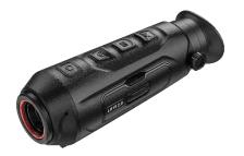
Featuring an impressive field of view spanning 43 meters, equipped with 384 sensors and boasting a 12 micrometer pixel pitch of high thermal sensitivity of NETD < 20 mK, the LH15 2.0 is designed to elevate the excitement of every forest hunter with a manual focus feature. Not only that, but field hunters will also appreciate its remarkable detection range, reaching up to 750 meters.
