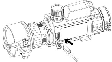
Figure 2-1 Cable Connection
