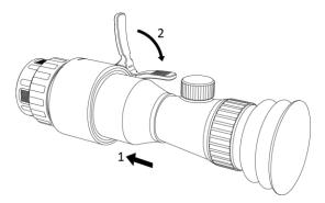
Figure 2-3 Install Daylight Scope
