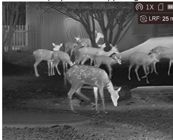
Figure 5-1 Distance Measurement Result
