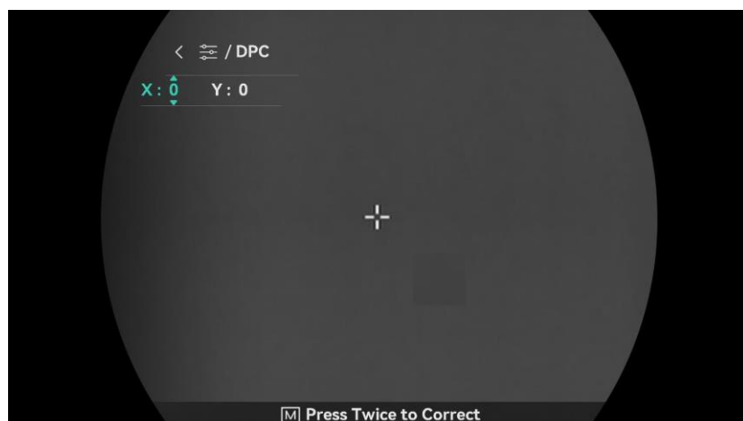
Figure 3-5 Correct Defective Pixel
