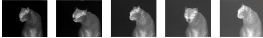
Figure 3-2 Adjust Brightness in White Hot Mode
