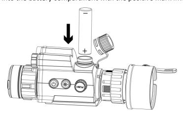
Figure 2-4 Install Battery
