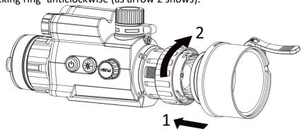
Figure 2-2 Install Adapter
