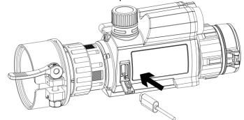
Figure 2-1 Cable Connection
