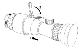
Figure 2-6 Install Daylight Scope
