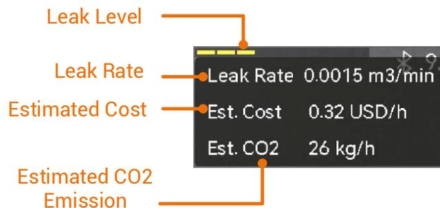
Figure 3-2 Gas Leak Estimation (Compressed Air)
