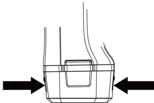
Figure 1-7 Remove Battery Base
