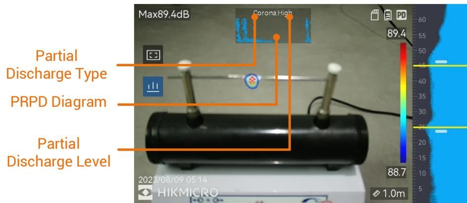
Figure 2-1 Partial Discharge Display
