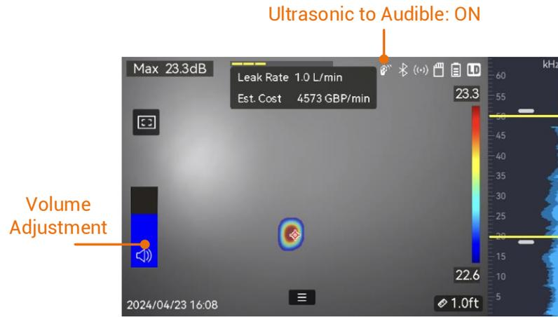
Figure 4-4 Ultrasonic to Audible and Volume Adjustment
