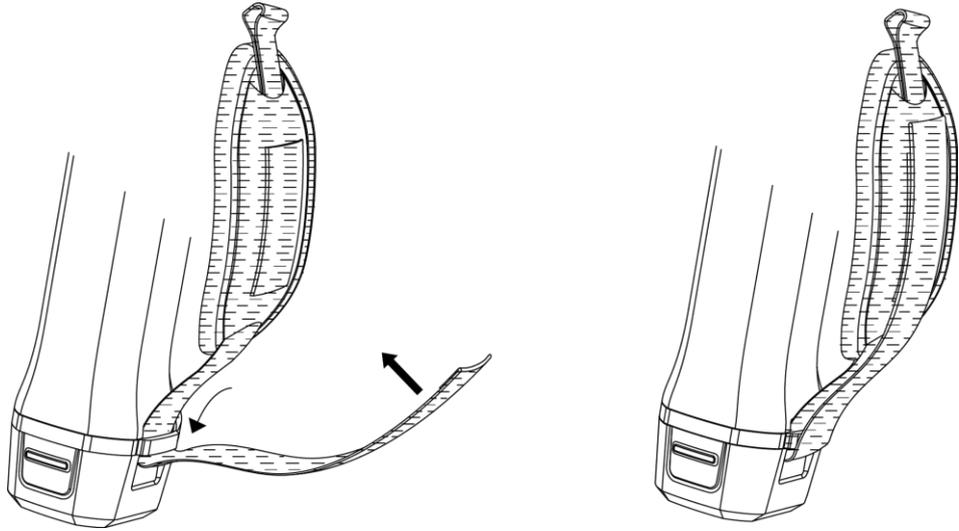
Figure 1-3 Secure Lower Part of Hand Strap
