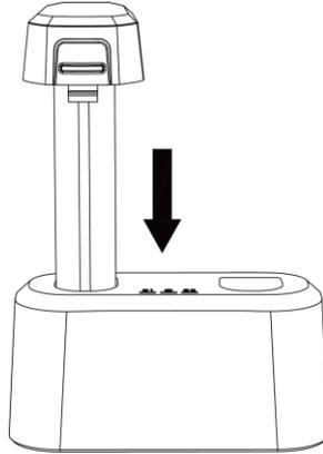
Figure 1-8 Charge Battery
