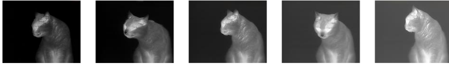
Figure 3-3 Adjust Brightness in White Hot Mode
