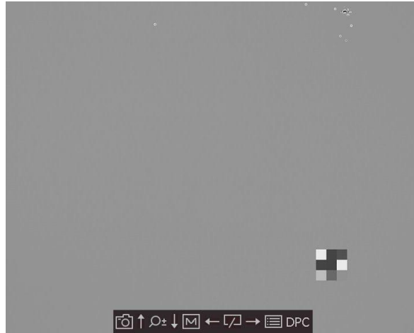
Figure 3-2 Correct Defective Pixel
