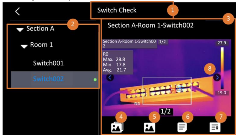
Figure 5-2 Route Inspection Work Flow
