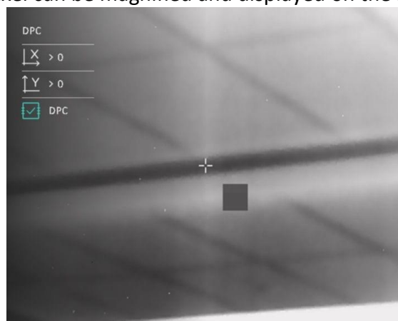
Figure 3-6 Correct Defective Pixel
