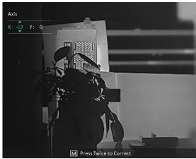
Figure 3-6 Correct Defective Pixel
