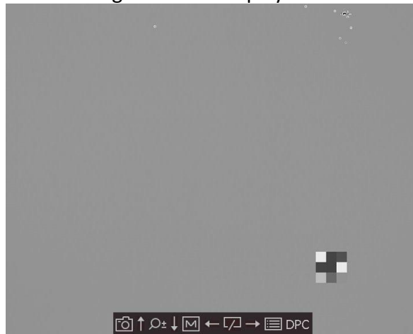
Figure 3-3 Correct Defective Pixel
