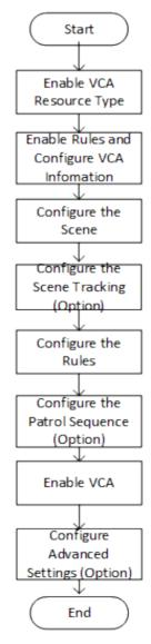
Figure 6-1 Flow Chart of Perimeter Protection Configuration
