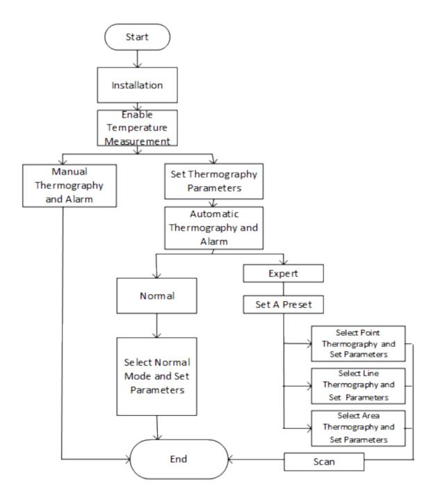
Figure 3-1 Thermography Configuration Flow Chart
