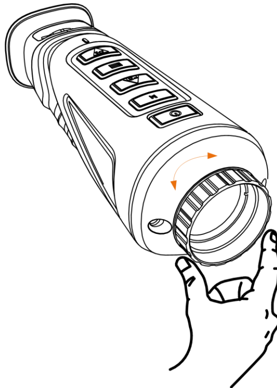
Figure 3-3 Adjust Objective Lens
