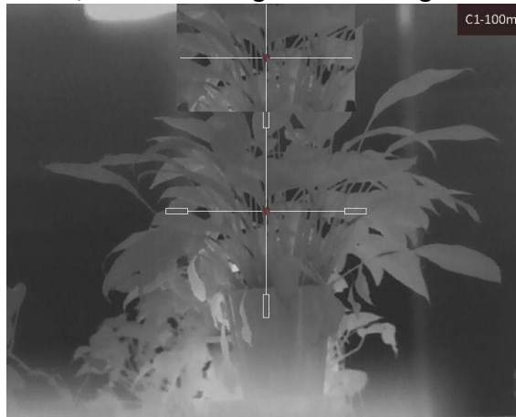
Figure 4-2 PIP Effect in Correcting Reticle
