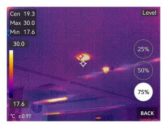
Figure 2-5 Adjust Optical-Thermal Ratio
