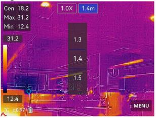
Figure 2-4 Adjust Parallax Correction
