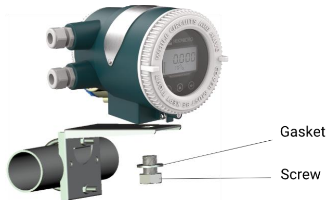
Figure 3-17 The Transmitter Is Secured to the Bracket With a Nut
