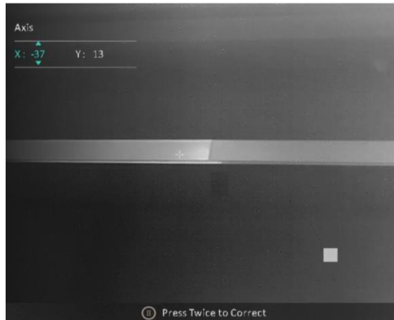
Figure 3-6 Correct Defective Pixel
