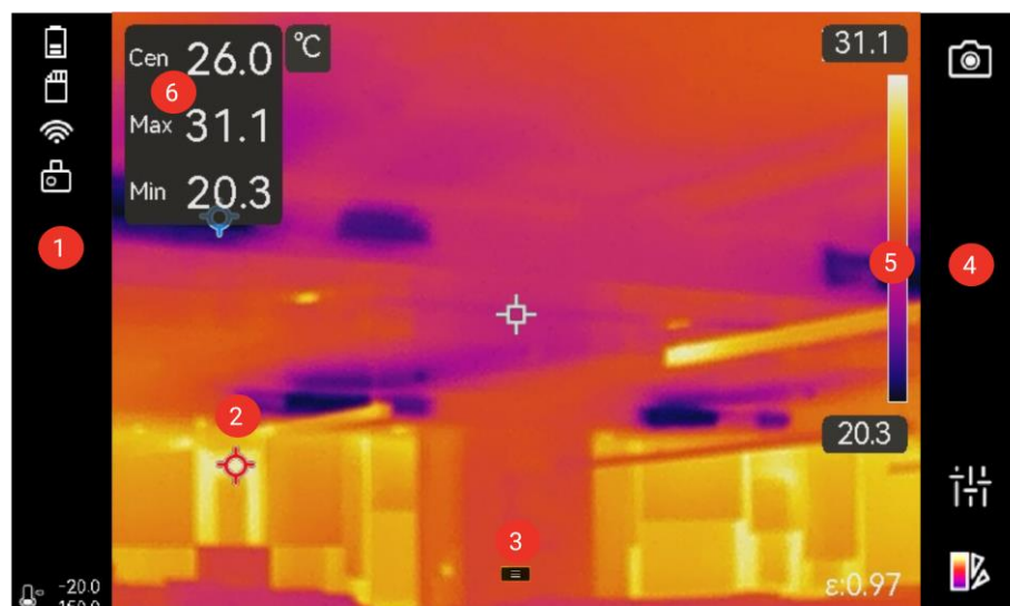
Figure 2-1 Live View Interface of Thermal Image Mode
