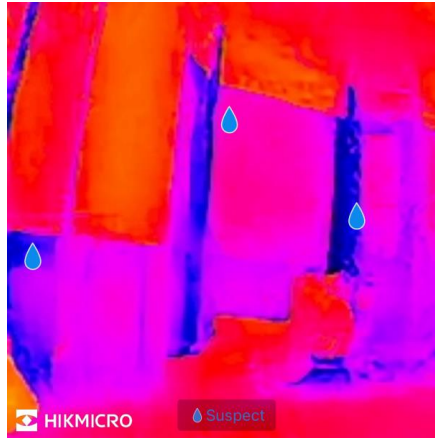
Figure 3-2 Water Leak Anomalies Recognition
