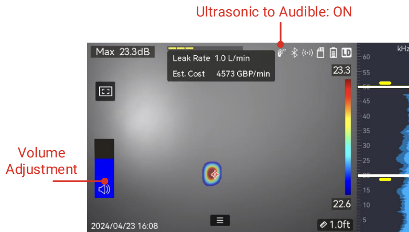
Figure 6-6 Ultrasonic to Audible and Volume Adjustment
