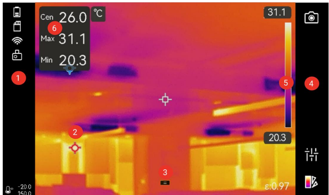
Figure 2-13 Live View Interface of Thermal Image Mode
